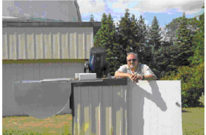
At this time both LX200 scopes can be run from the same heated office under the big dome. It will take some drift alignment to get the 10" scope better aligned to the pole but the scope is usable right now.
